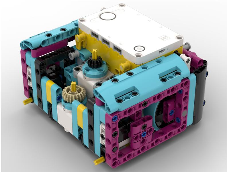
Actual Robot with cables: The cables should not protrude in the front so that the attachment can fit easily.
