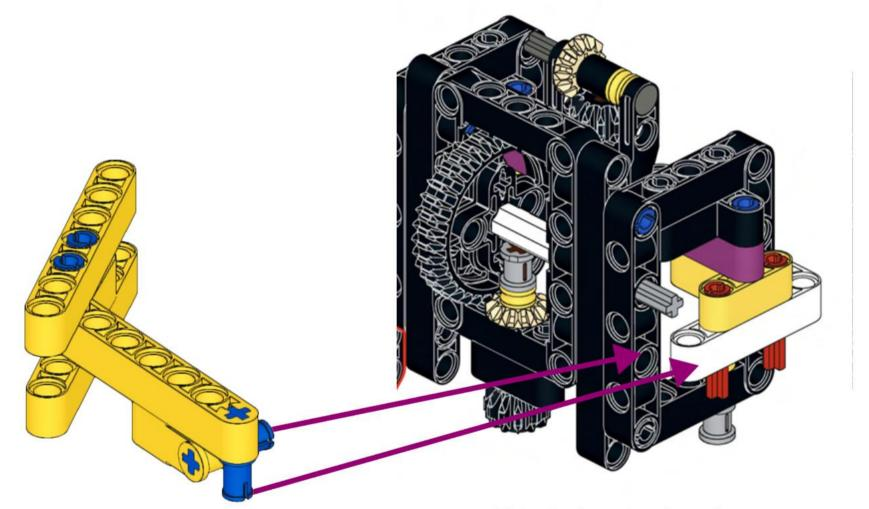
This attachment replaces the attachment arms starting on page 105 of Coop Bot. Connect the two blue pins as indicated above.
