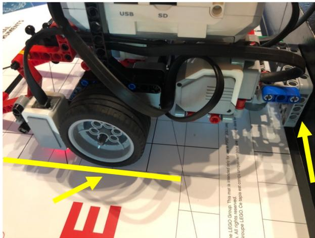
Align the robot flat against the South wall using the bumper
