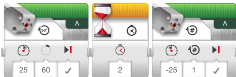
**Tip:** When activating a motor arm, it is important to start from the same position each time. Make sure the arm is down (as far as it can go) at the start of the program.
