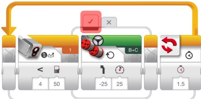
The color sensor is set to Compare → Reflected Light Intensity on Port 1
