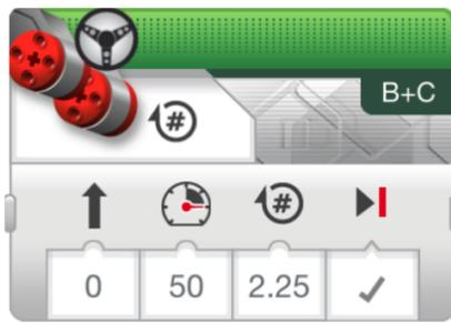
This is a Green Move Steering Block. It moves both motors at once and they are synchronized. The same block is used again after the line follower ends.
