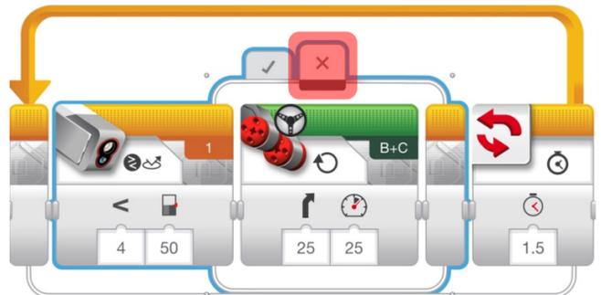
The robot turns right when False (ie. the threshold value read by the color sensor is greater than 50).
