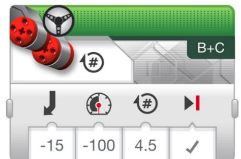
**Note:** This code moves backwards while turning so that your robot returns Home. This has been modified from the original code provided by FIRST which only returned to Launch.
